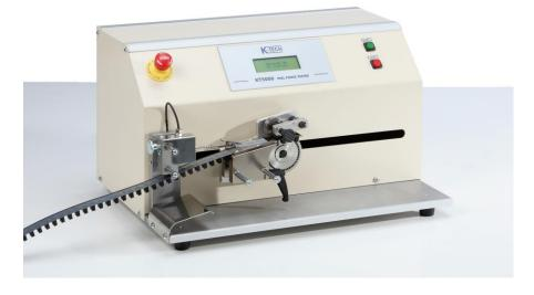
The peel force is a critical parameter for every user of Tape & Reel. If the peel force is too low, the cover tape will not stick on the carrier tape properly and the components may fall out of the pockets. A too high peel force will cause costly down times at the pick & place machines.
